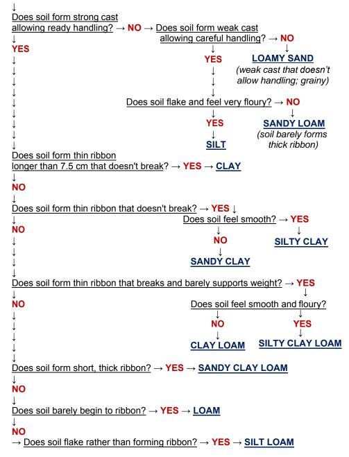
Created by Cole D. Gross, Copyright @ 2018  $\mid$  Soil Hand-Texturing Test
